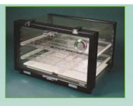
gasketed door with two metal hinges, two latches and door handle. Includes desiccant tray and dial hygrometer. The door opening is 45 x 25cm (17% x 10"), inside depth is 34cm (131/4").
